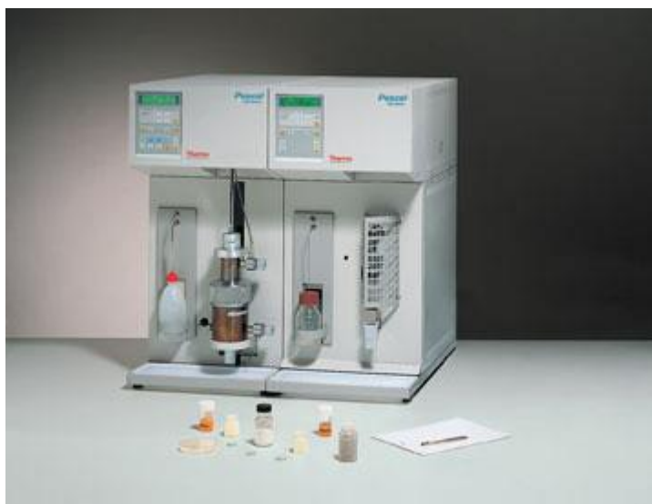
Figura 2.16. Porozimetrul cu mercur ( http://www.porexpert.com/Porosimetry.html )
